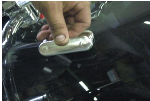
G) securly tight the nuts in to the windshield bracket
