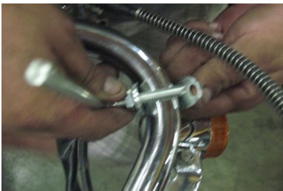
D) Wrap handle bar with clamp and insert the arm brackets
