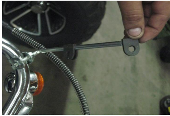
E) Install the windshield holder to the arm bracket
