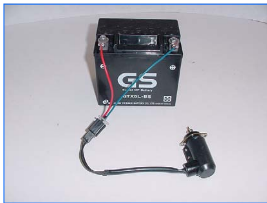
12 volts applied to the choke cylinder
