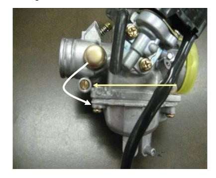
**NOTE**: At Higher altitude, you need to adjust the THROTTLE CONTROL (YELLOW ARROW). To properly adjust THROTTLE CONTROL, turn COUNTERCLOCKWISE 2 times. DIRECTION OF WHITE ARROW.
